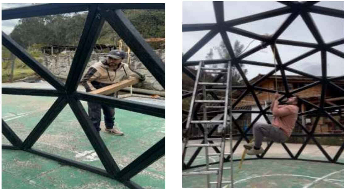
Figure 20 Impact Test on Nodes and Experimental Test to simulate a Vertical Load.
