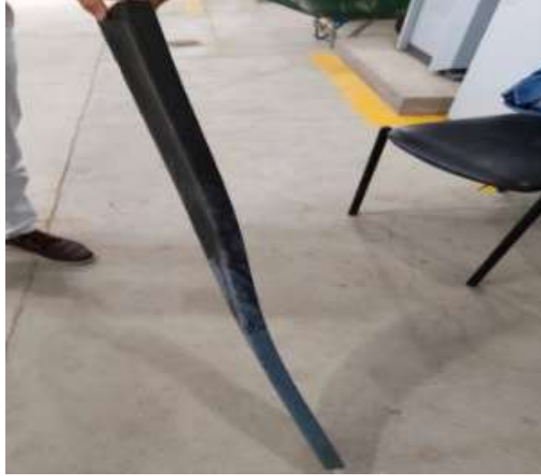
Figure 9 Example of Lateral Torsional Buckling in a Tested Structural Element
