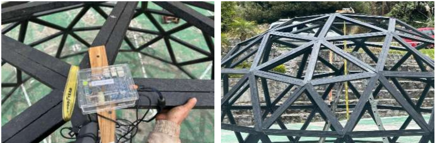
Figure 19 Installation and location of Raspberry Shake 3D.
