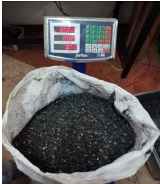
Figure 12 Shredded Type 5 Plastic (Polypropylene)
