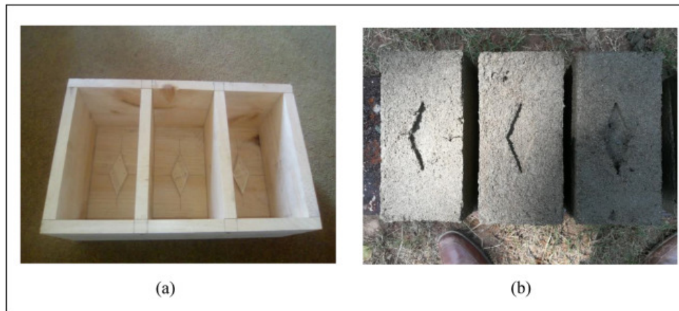
FIGURA 1.5: Boardcrete. Tomado de: Mechanical properties and durability of boardcrete block prepared from recycled cardboard, Ahmad, Adil, Khalil, & Rahman, 2021.
